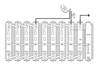
Example os SRF headend of eight clear digital satellite TV programs; four programmes access via a down lead cable and other four ones via another. Contains 8 receives, 1 amplifier and 1 power supply, all fixed on 2 base-plates.
